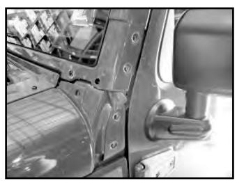
2. Place the Stainless Steel Windshield Bracket in place and start the top screws on the side and front to hold the bracket in place.
