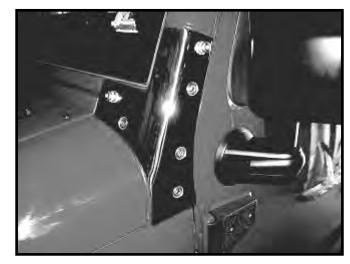
3. Start all remaining screws. Once all screws are in place, tighten them using a T-40 Torx wrench. Repeat steps 1-3 for the other side.
