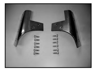
1. Remove the original windshield brackets using a T-40 Torx wrench.
