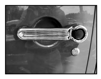
4. Remove plastic backing film from the affixed two sided 3M<sup>®</sup> tape on the inside of one Button Cover. Center the Button Cover on door handle button and apply pressure to secure to vehicle.
