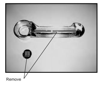
3. Position Door Handle Cover on door handle and apply pressure to secure to vehicle.
