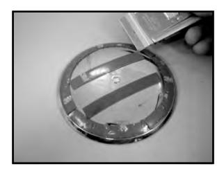
Position Door Recess Guard in the door recess. Peel tape backing from perimeter tape. Apply pressure to all tape attachment areas to ensure good adhesion.
