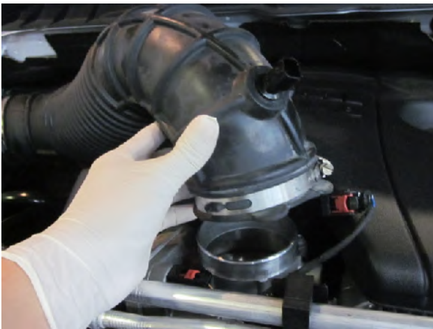
e) Detach the factory air intake hose from the throttle body.
