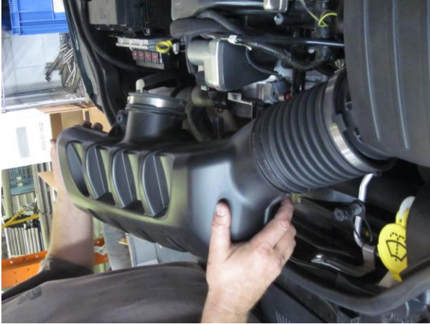
g) Remove the air inlet hose from the engine bay.
