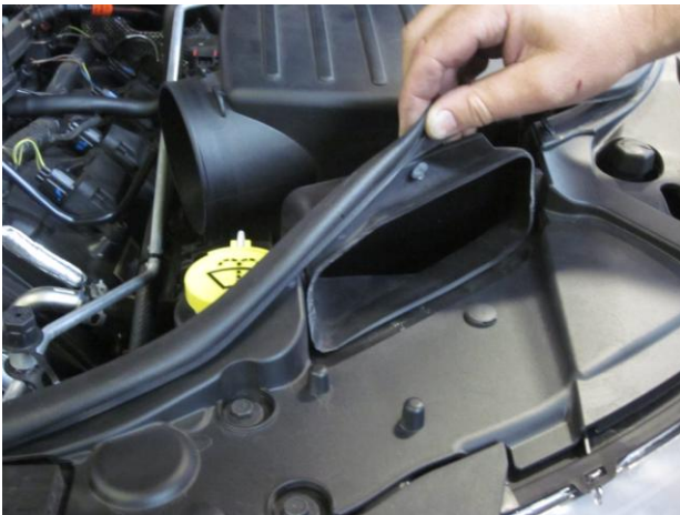
i) Detach the air inlet duct from the rubber edge trim.
