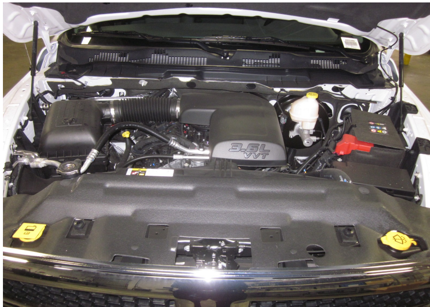
a) The stock air intake system should look like this.
