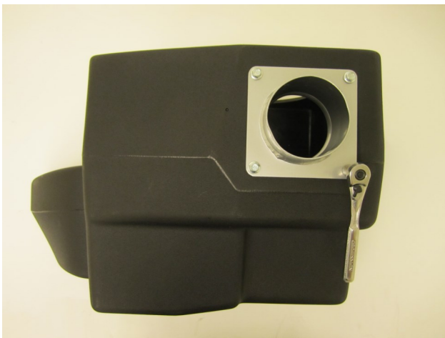
c) Attach the flanged air filter adaptor to the MOPAR air box with four (4) M6 bolts provided to 7 N.m (62 in/lb).
