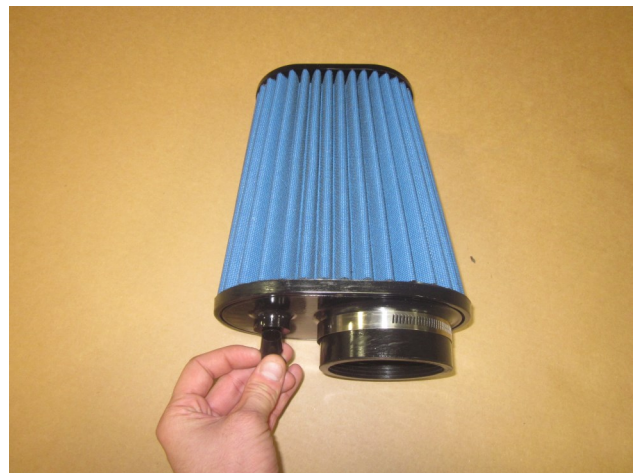
d) Install the supplied adaptor plug into the hole on the air filter.
