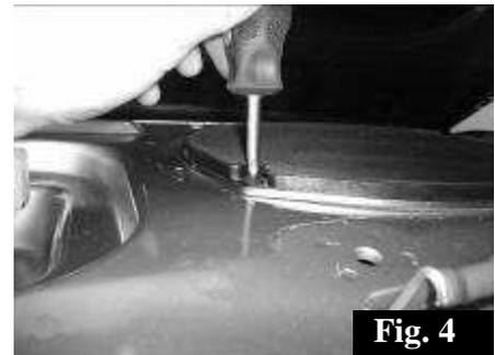
7. Install the upgrade speakers replace the screws and tighten.
