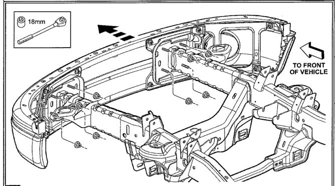
1 Remove (8) front bumper mounting nuts. Remove the bumper.
