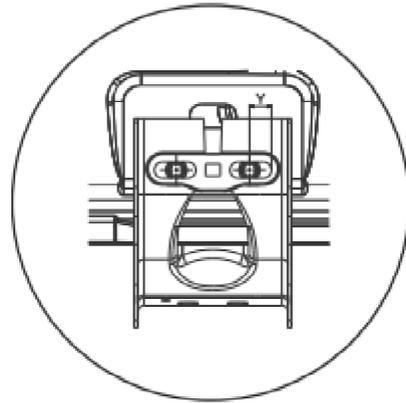
Using 2 M8 fasteners (item B) loose assemble the bracket removed in step 3 and mark the drill locations in the pinch weld. All measurements will be taken from the rear most edge of the rear slot on the upper part of the bracket to the center of the corresponding rivnut.
