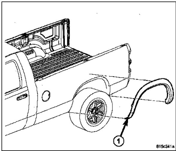
5. Install the push-pin (1) first for correct flare positioning. Install the six screws (2) in sequence starting from the center and proceeding outward. For a correct fit, hold the flare tight against the fender as the screws are tightened. Tighten to 2.3 N·m (20 In. lbs.).
