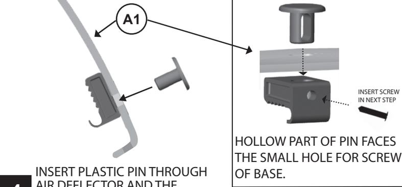
**4** INSERT PLASTIC PIN THROUGH AIR DEFLECTOR AND THE FASTENER BASE. (X5)
