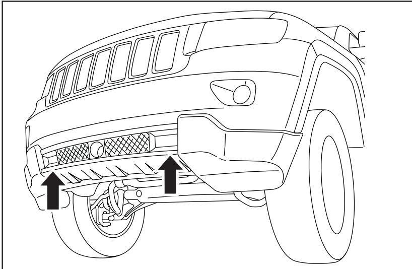
2. Remove lower front cover plate, inner bumper trim panel and lower front bumper trim panel.
