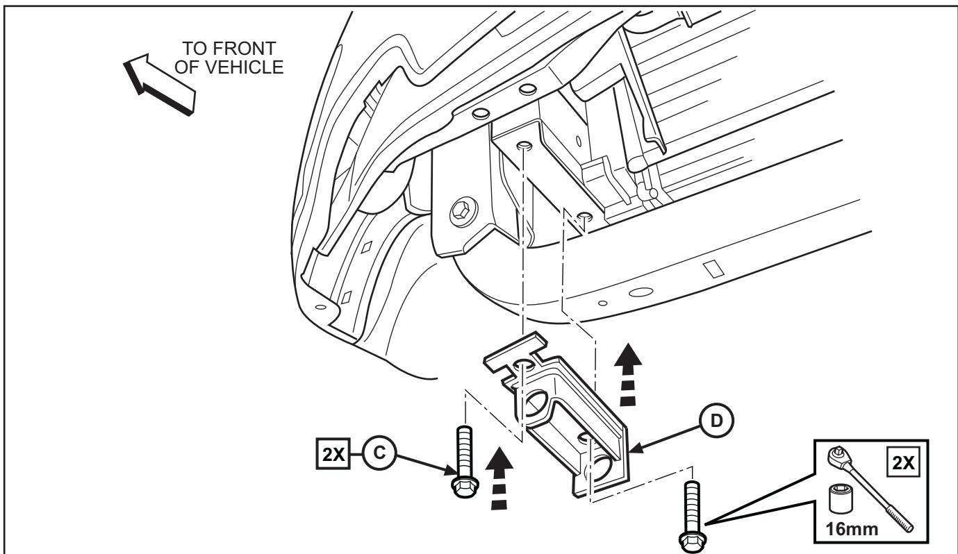
4. Install spacer bracket, two-sided tape, (2) spacers, cover plate, and tow hook as shown using (2) 18mm bolts, (2) washers (2) nuts and (1) 30mm nut provided. Tighten 18mm bolts to 47 Nm (35 ft. lbs.). Tighten 30mm bolt to 25 Nm (18 ft. lbs.).
