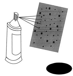
GENEROUSLY COAT ENTIRE SURFACE OF TEXTURE PAD. (THIN LAYER OF LITHIUM GREASE MAY BE USED IN PLACE OF MOLD RELEASE)
