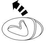
REMOVE THE SLUG OF MATERIAL INSIDE THE CUT LINE.
