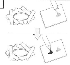
PRIME THE MIXING TIP AWAY FROM THE REPAIR AREA TO ENSURE PROPER MATERIAL MIXING
