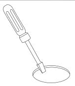
USE A FLAT HEAD SCREWDRIVER TO CLEAN REMAINING DEBRIS FROM THE REPAIR AREA.
