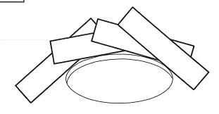
TIGHTLY MASK AROUND THE REPAIR AREA WITH ANY GENERAL MASKING TAPE.
