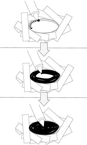
TIGHTLY MASK AROUND THA REPAIR AREA WITH ANY GENERAL MASKING TAPE.
