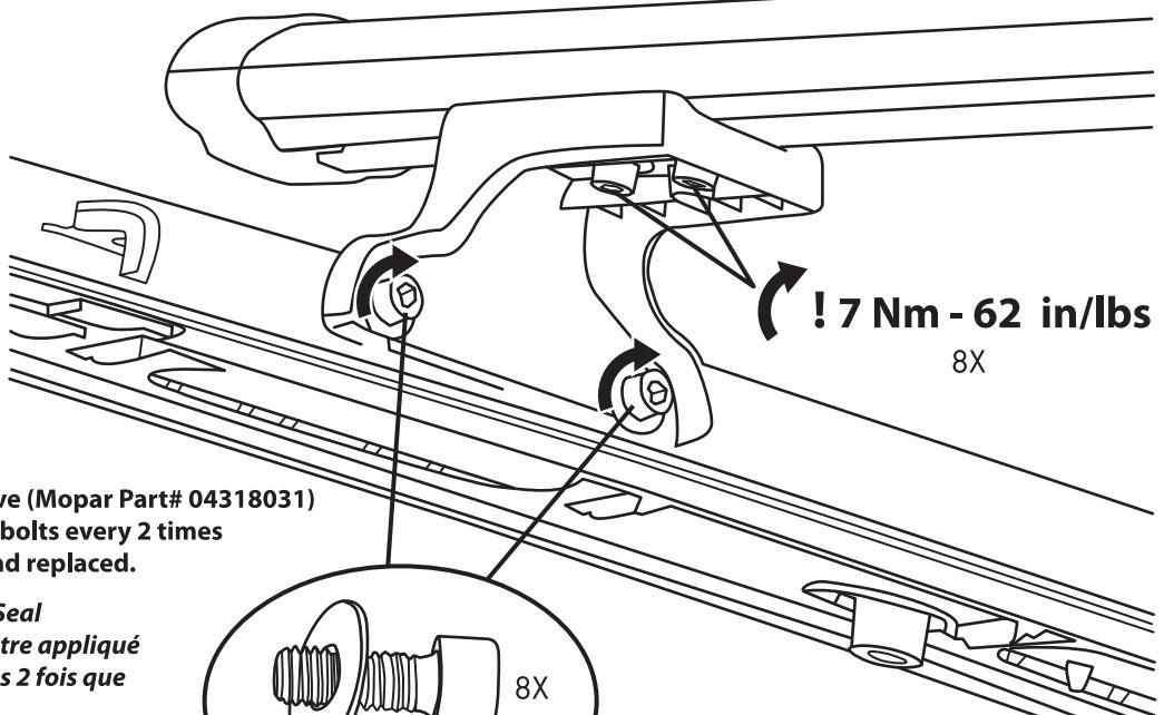
**ATTENTION:** Lock & Seal Adhesive (Mopar Part# 04318031) must be reapplied to threads of bolts every 2 times the rack assembly is removed and replaced.
