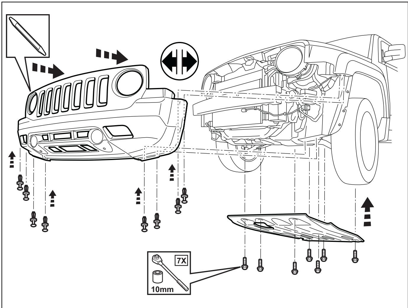
6. Reinstall (4) fasteners along top of fascia panel.
