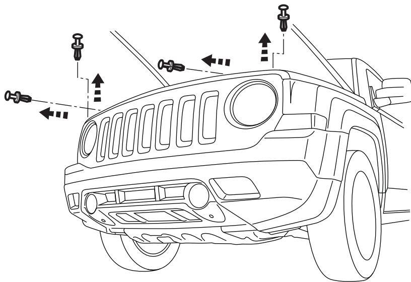
3. Raise vehicle on hoist. Remove lower front cover plate. Disconnect wheel well clips and remove remaining fasteners as shown. Disconnect electrical connectors and remove fascia panel.
