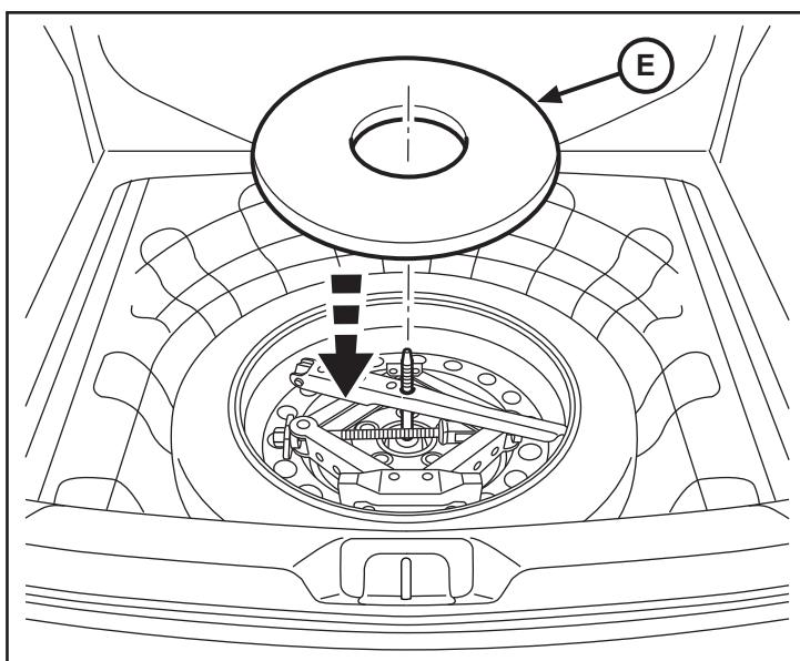
7. Firmly secure the spare tire and jack assembly with the wing nut. Do not over tighten.
