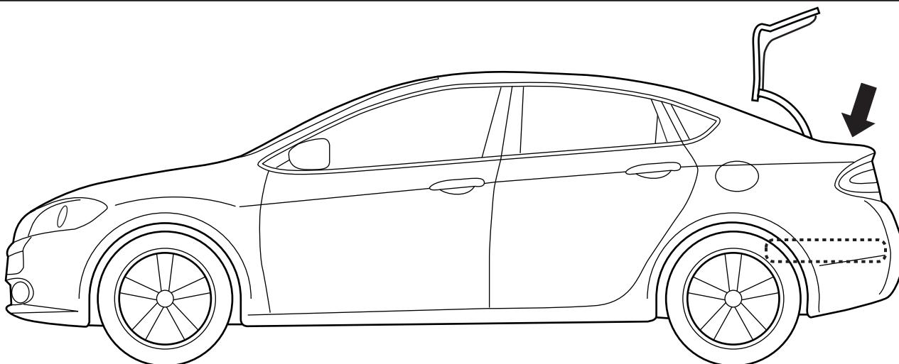
2. Open the trunk. Remove the floor access panel.
