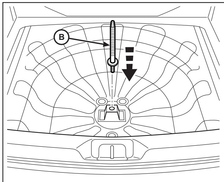
4. Place the spare tire into the trunk cavity making sure the mounting shaft comes up through the center of the tire.
