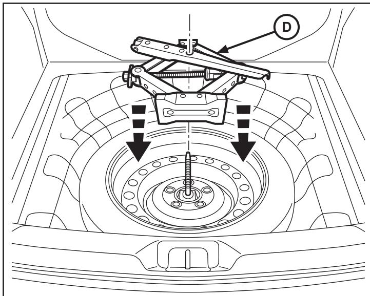
6. Place the protective cover disk into position over the jack.
