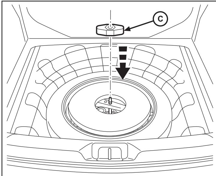
8. Reinstall the floor access panel inside the trunk.
