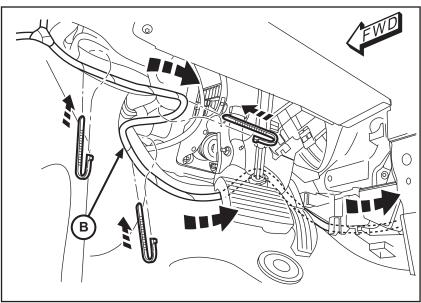
40. Use a pry tool to carefully remove the cover panel under the glovebox. Pull down the carpeting in the footwell.
