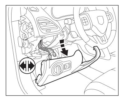
6. Use a pry tool to carefully remove the cover panel under the dash. Disconnect one (1) plug.
