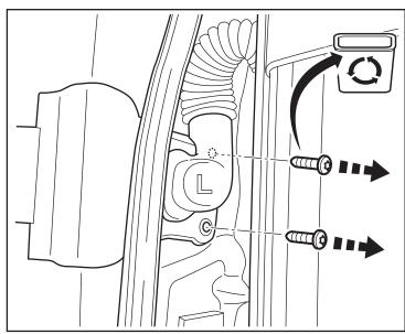
16. Remove four (4) T-25 Torx screws from the speaker. Pull the speaker out and unplug the electrical connector. Remove the speaker.
