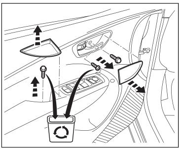
10. Use a trim stick to pry up the switch module from the armrest. Disconnect two (2) plugs.
