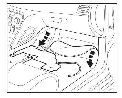
41. Route the new body harness along the existing harness under the glovebox and out towards the passenger door. Secure with cable ties.
