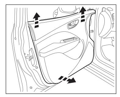
12. From inside the panel, use a pry stick to press the release tab at the back of the door handle assembly. Remove the handle assembly. Completely remove the door panel and set aside.
