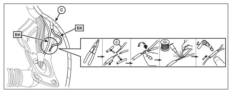
25. Feed the end of the new mirror harness through the boot tube and out towards the A-pillar connector as shown.
