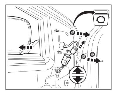
15. Remove two (2) fasteners from the wiring boot bracket at the bottom of the front inside door edge.
