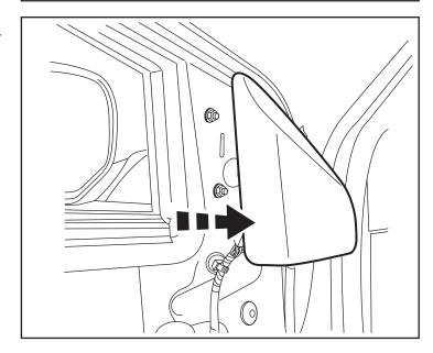
14. Disconnect the mirror plug. Remove three (3) 8mm hex bolts from the inside mirror mounts. Remove the mirror assembly.
