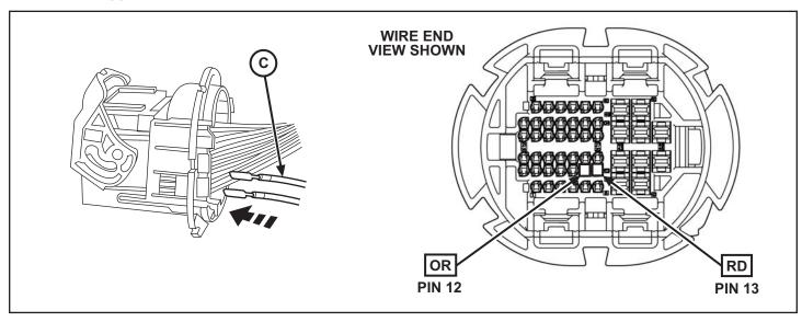
28. The body harness is designed to connect at both sides of the vehicle with a T-harness that will reach up to the BCM. Locate the shorter section of the body harness relative to the T-harness. Position the two wire ends near the 48 way connector inside the driver footwell.
