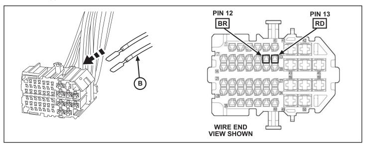
31. Looking up inside the dash, locate the C4, 60 way connector in the lower left corner of the BCM.
