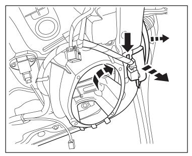
18. Carefully pull back the wiring boot cover at the A-pillar by the door hinge. Using a right-angle pick tool, press in on four (4) tabs to release the 48-way connector.
