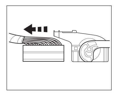
35. Position the three wire ends from the shortest section of the body harness near the back of the connector. Insert the harness wiring as follows:
