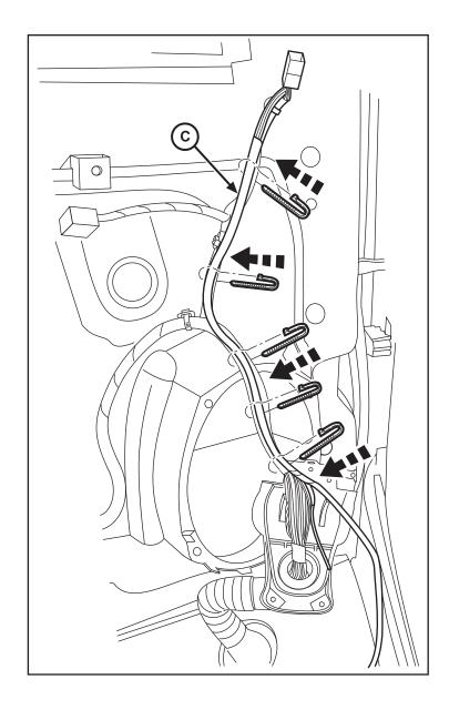
24. Locate the black wire in the harness on the back of boot bracket. Verify that this is the ground wire located in pin 49 of the door/boot connector. Splice the black pigtail wire from the new mirror harness to the black wire behind the boot bracket.
