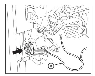
29. Use a pry tool to remove the terminal locks from the left and right sides of the 48 way connector.
