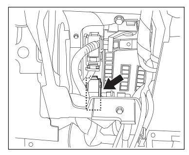
32. Press in on the locking tab and flip the blue retaining lever open to release the 60 way connector.
