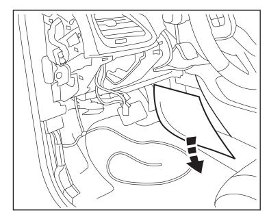
39. Route the new body harness along the existing harness under the dash and secure with cable ties. Be sure the harness passes behind the brake and accelerator pedals without causing any interference. Feed the end of the harness through the center stack and out to the passenger side footwell.
