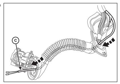
26. Use a pry tool to remove the terminal locks from the top and bottom of the A-pillar connector.
