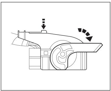
33. Carefully pull the 60 way connector down into the footwell.
