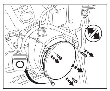
17. Carefully pull away the seal welt at the front edge of the door. Reach inside the speaker opening and press the mounting clip to release the wiring boot bracket from the front of the door.
