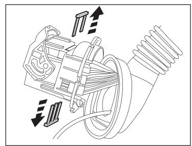
27. Position the two wire ends near the back of the connector. Insert the harness wiring as follows: Orange wire into Pin 12 Red wire into Pin 13
