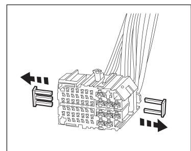
30. Position the two wire ends near the back of the connector. Insert the harness wiring as follows: Brown wire into Pin 12 Red wire into Pin 13
