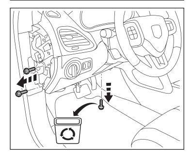
5. Carefully pull panel down. Disconnect four (4) plugs from the back of the panel. Press in on the retainer tab to remove the hood release latch assembly. Completely remove the panel.
