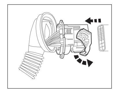
20. Looking at the back of the harness boot bracket, release the five (5) tabs to remove the back cover.
