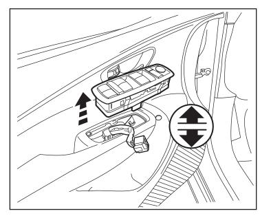
11. Carefully pry the bottom of the door panel outward to unfasten clips. Lift the panel upward to release it from the door. Disconnect all electrical connectors from inside door panel.
