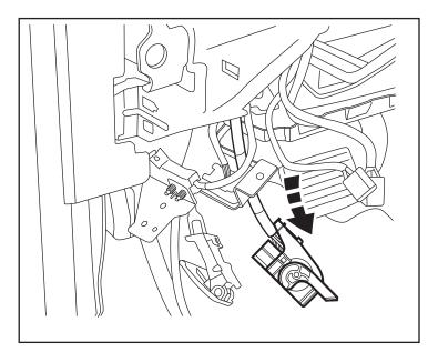
34. Press in on the release tabs at the back of the 60 way connector and slide the plug out from the outer casing.
