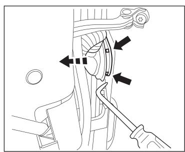
Press in on the locking tab and flip the retaining lever open to release the connector. Pull the connector and wiring boot out from the front door edge.
