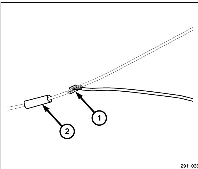
30. Using a crimping tool (1), crimp the splice clip and wires together.
