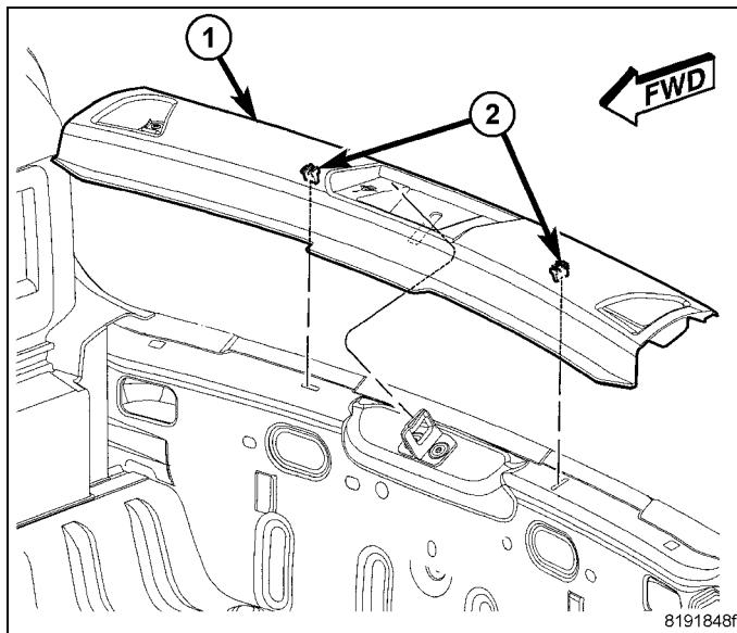
61. Position the cargo floor into the vehicle and engage the rear pivots.
