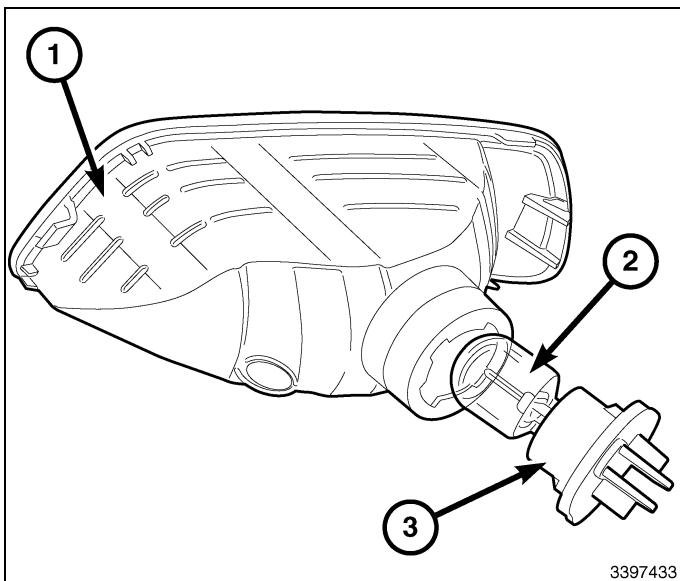
52. Align and position the fog lamp (1) into the opening. Push the fog lamp in to engage the retaining tabs.
