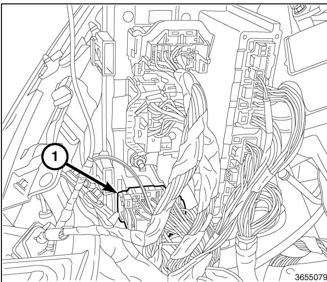
26. With Connector L (1) removed from the TIPM, locate the white/yellow wire (2) in cavity 5.
