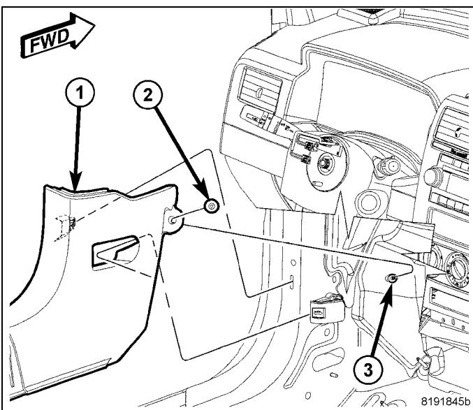
65. Position the driver door scuff plate (3) into back into place over the scuff (1) and seat the retaining clips fully.
