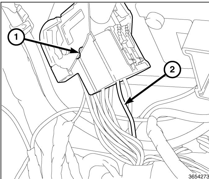
28. Measure approximately 4 inches from the pin of the white/yellow wire and mark accordingly for splice location and cut the wire.
