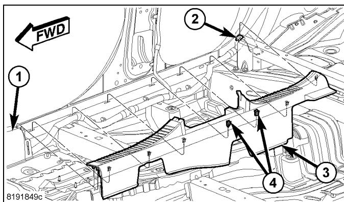
3. Remove the fastener (2) and release the retaining clip.
