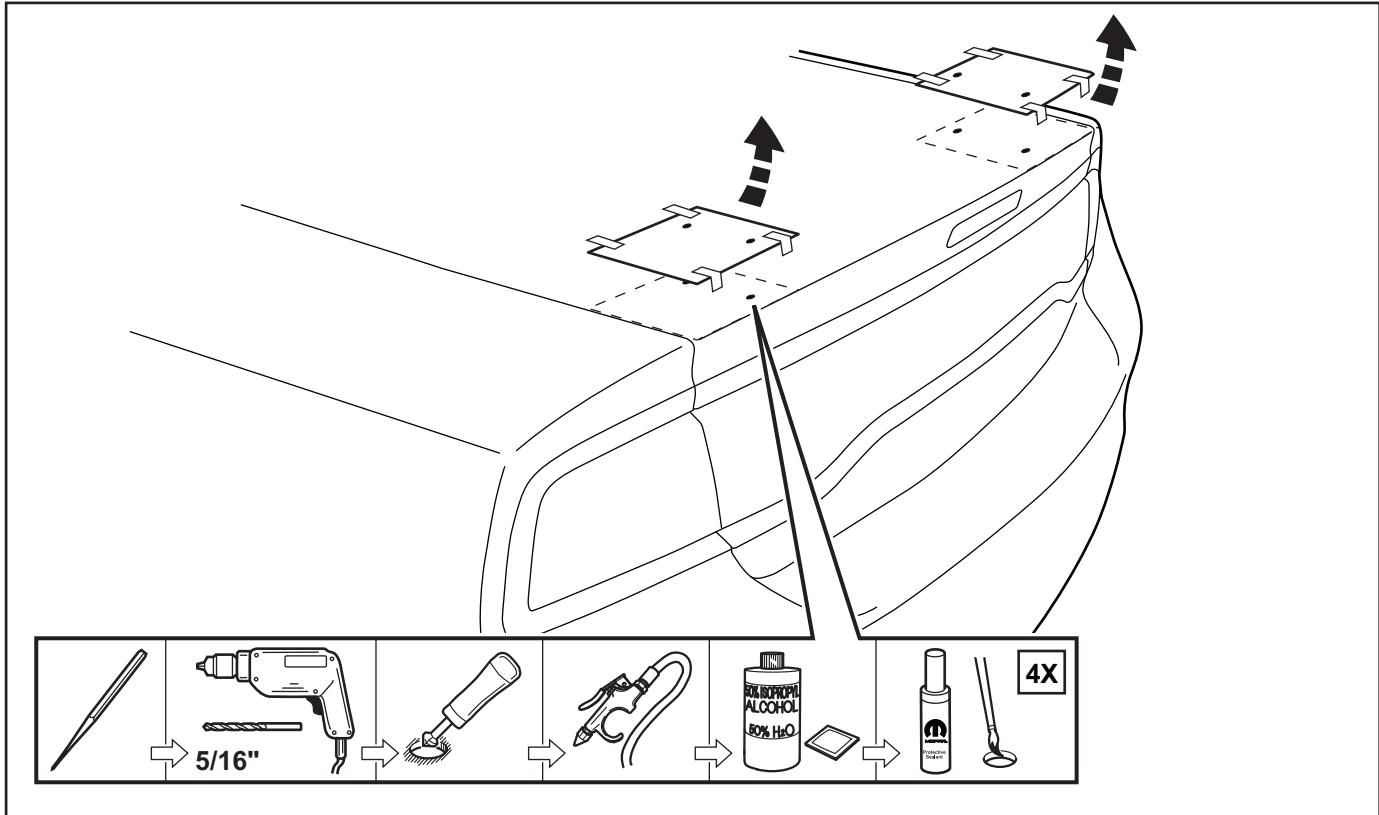
7. Place spoiler into mounting holes and hold in position. Open trunk lid and attach (4) 10mm mounting nuts to spoiler from the inside. Tighten to 6 Nm (4.5 ft. lbs.).
