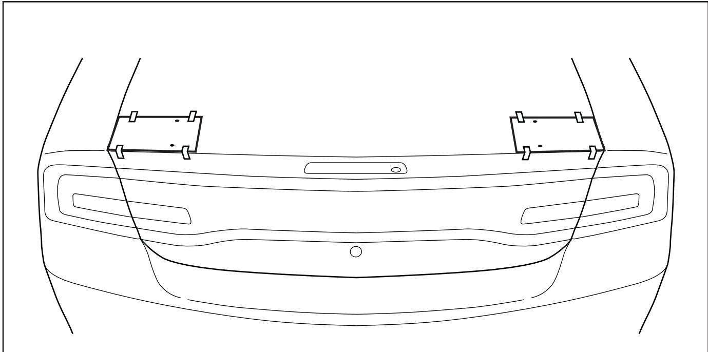
5. **IMPORTANT:** Before marking and drilling the mounting holes, verify the measurements as they are marked on the template with a ruler. Also make a visual check by positioning the spoiler on the trunk lid and double-check the hole positions with the sheet metal openings inside the trunk lid.
