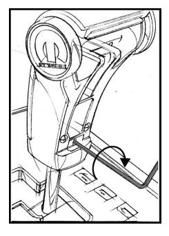
5. Once the shifter handle is in place, tighten the set screw located at the bottom of the shifter handle. (Torque to 13 inch-pounds)
