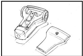
4. Place the shifter handle on the shaft and using a screwdriver or similar tool placed inside the handle (CAUTION - NOT ON THE COVER) and a rubber mallet - tap into place.
