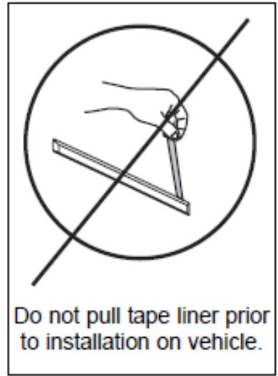
Do not pull tape liner prior to installation on vehicle.
