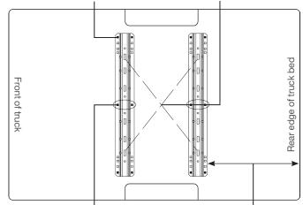
Each mounting rail must have a bolt in either of the marked holes. Check for obstructions before drilling Rear edge of truck bed to rear edge of mounting rail
