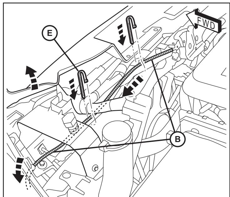
8. Route the switch harness (B) along the existing vehicle harnesses on the driver side and back towards the rear of the engine compartment. Tuck the harness behind the fuse box as shown.
