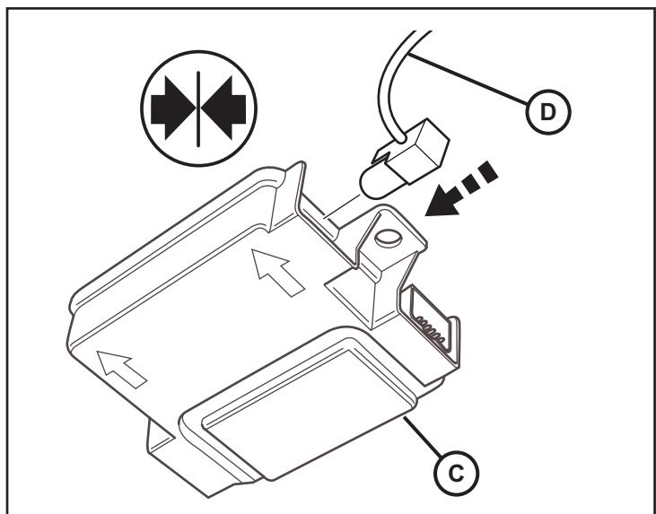
26. Place the new RF Hub Module (C) into position. Secure the RF Hub Module to the roof with two (2) fasteners and reconnect all harness connectors.
