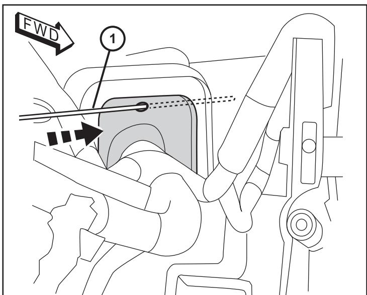
14. Secure the end of the harness to the fish wire with tape. Pull the end of harness (B) through to the inside driver footwell. Apply RTV sealant to the hood switch wiring convolute and pull the wiring into the nipple to seal the wiring at the nipple.
