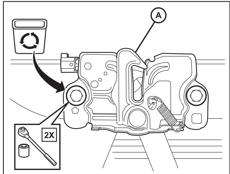
**NOTE:** A factory installed switch harness may be present. If so, detach the connector, route it under the crossmember and plug it in to the hood latch assembly, then proceed to Step 20.
