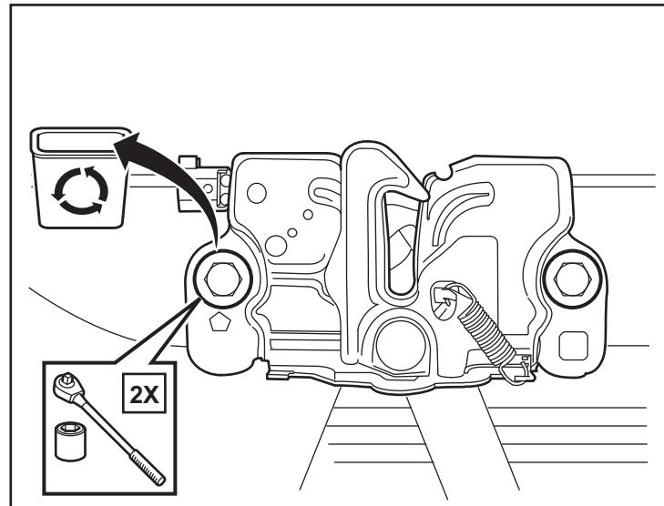
4. Carefully pry back the radiator cover panel. Disconnect and remove the hood latch release cable. Remove the hood latch assembly.
