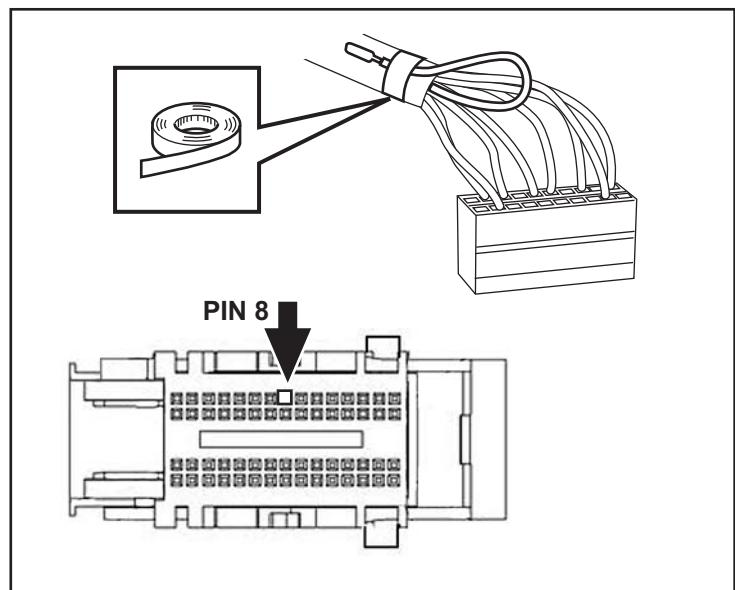
18. Insert the tab wire connector from switch harness (B) into Pin 8 on the connector.
