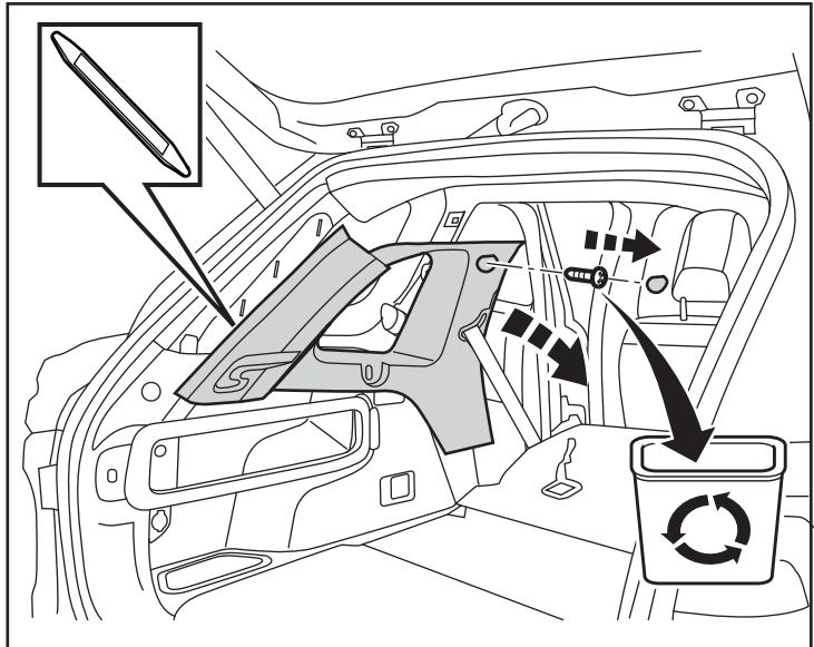
22. Carefully pry down the back edge of the headliner at the top of the cargo area.
