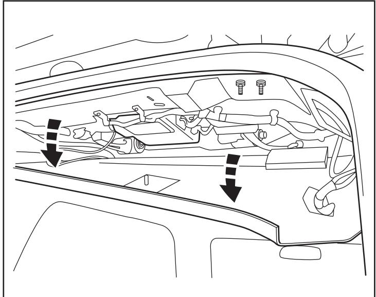
23. Locate the existing RF Hub Module on the roof center area. Disconnect all harness connectors. Remove two (2) fasteners. Remove the RF Hub Module.
