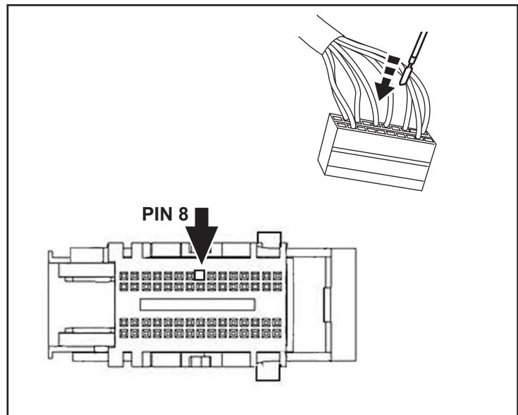
19. Reinstall the outer casing on the connector. Plug all connectors back into the BCM.
