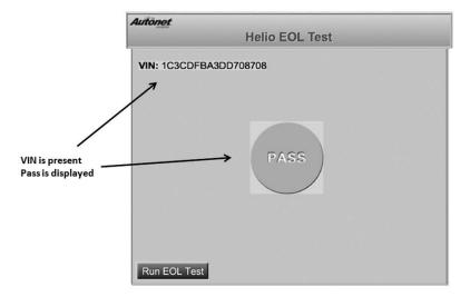
If both parts of the EOL test pass, then EOL testing is complete. Otherwise, continue to Step 12.
