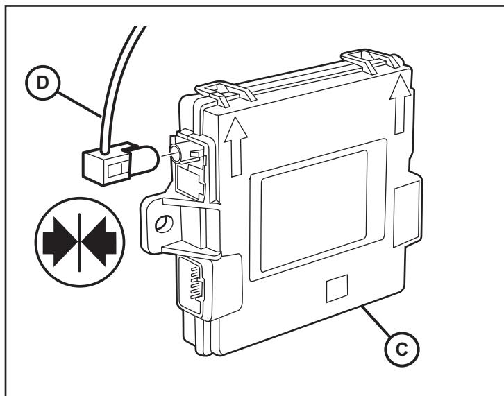
37. Place the new RF Hub Module (C) into position. Secure the RF Hub Module to the wall with two (2) hex nut fasteners (F) and reconnect all harness connectors.
