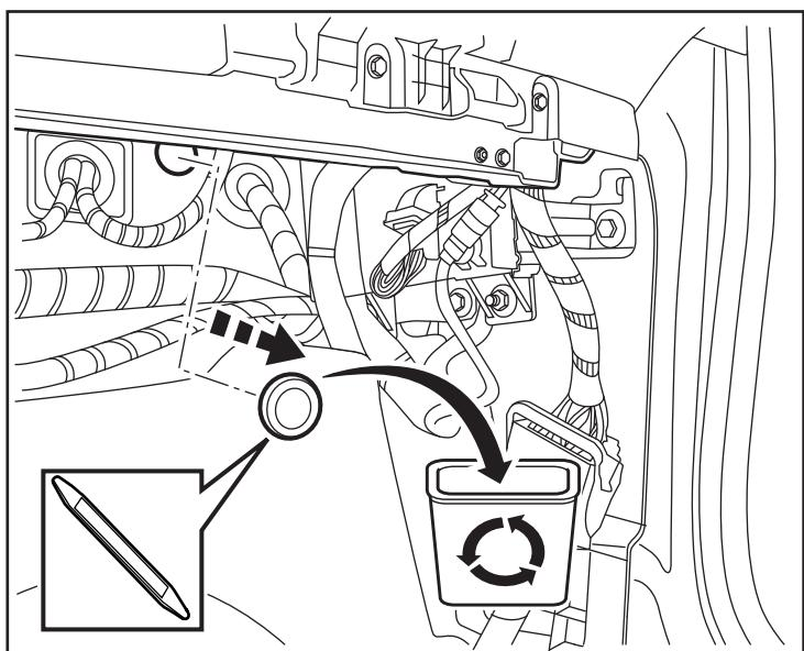
20. From inside the engine compartment, feed the switch harness (B) through the grommet hole and into the passenger side footwell.
