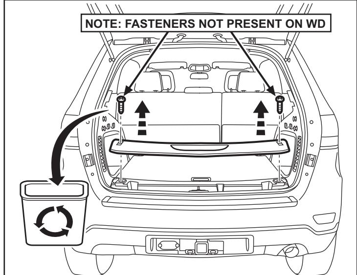
31. Remove the cargo deck cover panel from the vehicle.
