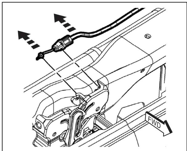
5. Reconnect the hood latch release cable to the back of new hood latch assembly. Position the new hood latch (A) with the alignment marks and secure with two (2) hex bolts. Tighten bolts to 11 Nm (8 ft. lbs.)
