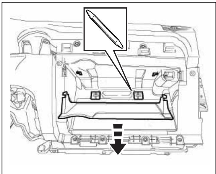
18. Remove four (4) fasteners from the bottom edge and two (2) fasteners hidden in rubber bumpers on the top edge of the glovebox surround. Disconnect one (1) electrical connector on the right side of the glovebox surround. Remove the glovebox surround from the vehicle.
