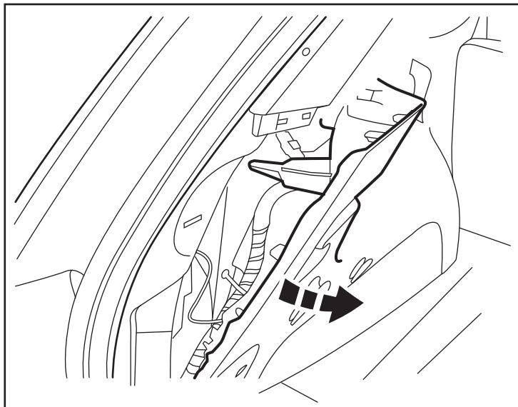
35. Locate the existing RF Hub Module on the driver side pillar of the rear hatch area. Disconnect all harness connectors. Remove two (2) hex nuts fasteners. Remove the RF Hub Module.
