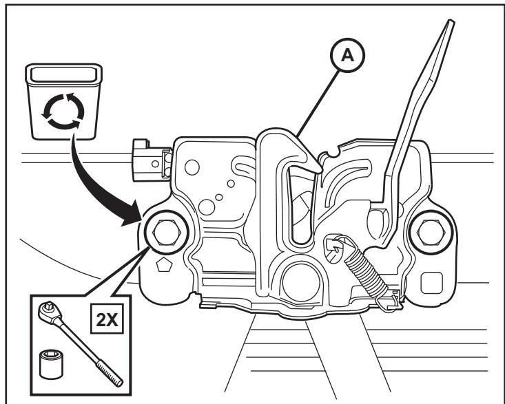
**NOTE:** A factory installed switch harness may be present. If so, detach the connector, route it under the crossmember and plug it in to the hood latch assembly, then proceed to Step 28.
