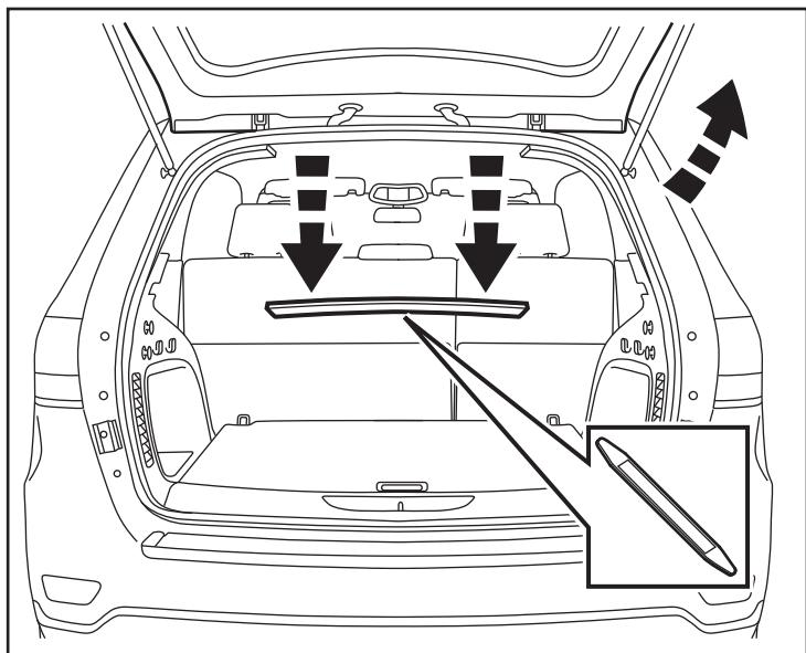
29. Carefully pry off the upper trim panel from the driver side rear hatch area. Release the safety strap from the back of the panel and remove the panel from the vehicle.
