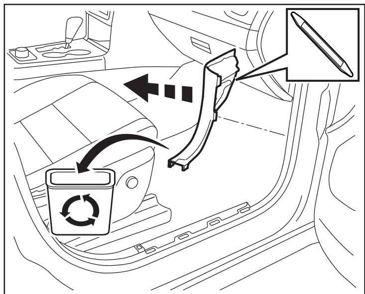
14. Use a pry tool to remove two (2) fasteners from the cover panel under the glovebox. Disconnect the two (2) electrical connectors on the back side of the cover panel. Remove the cover panel.
