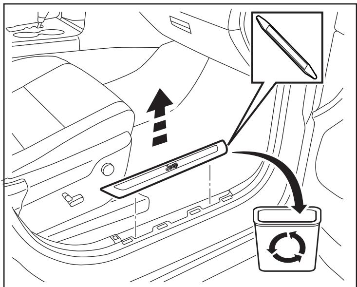
13. Remove weatherstrip near the outer footwell trim panel, then carefully pry off the outer footwell trim panel.
