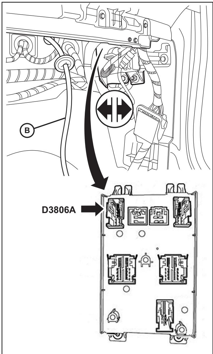
23. Isolate the top left connector plug from the BCM. Press in on the release tabs at the back of the connector and slide the plug out from the outer casing.
