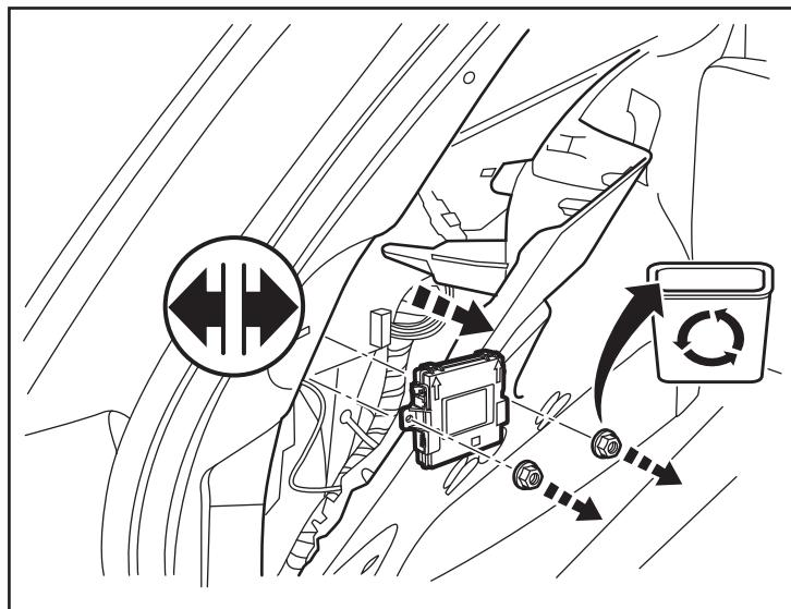
36. Plug the Antenna Module cable (D) into the new RF Hub module (C).
