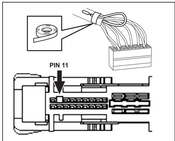
25. Insert the tab wire connector from switch harness (B) into Pin 11 on the connector.
