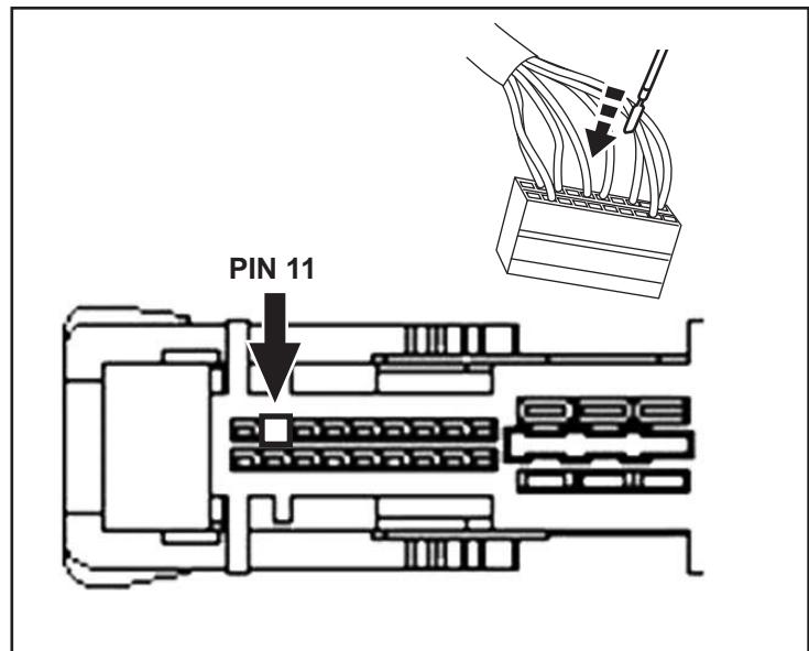
26. Reinstall the outer casing on the connector.
