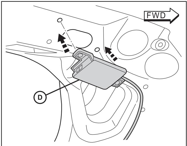
41. Secure the antenna module harness (D) along the existing vehicle harnesses inside the rear pillar with cable ties (E).
