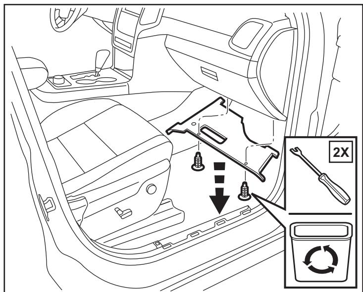
15. Using a trim stick to remove the passenger side end cap.
