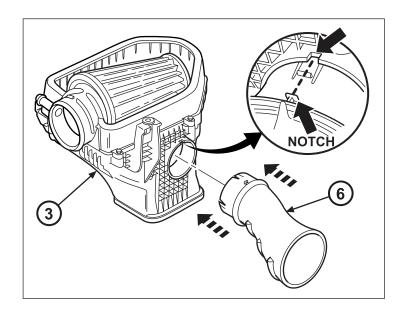
21. Install airbox assembly (3), tilting the headlamp duct (6) down first fitting into the headlamp deflector opening as shown.
