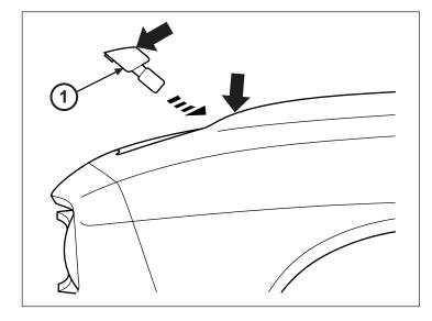
9. Install double stud (9) into center hood prefab hole opening, snap to lock in place.
