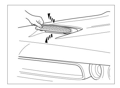
7. Remove red strip from bottom of hood scoop bezel adhesive tape (1).
