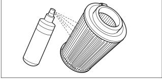
**2. APPLY CLEANER**Spray the air filter with MOPAR Filter Cleaner and allow the solution to soak in for about 15 minutes.
