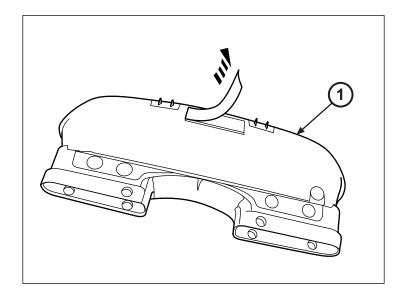
8. Angle the bezel adaptor assembly (1), starting from the top and slide into hood scoop opening. Press down on the hood scoop bezel (1) gently rocking it into place.
