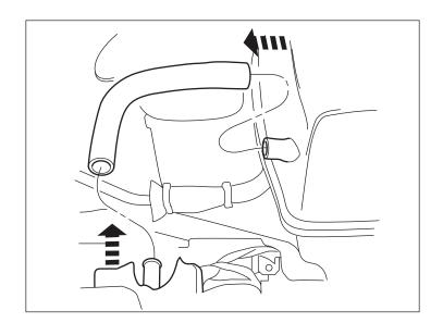
17. Loosen band clamp on air inlet hose to airbox with a 8mm socket. Remove airbox mounting bolt with a 8mm socket, save bolt for reinstallation.
