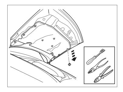
4. Using "painters tape" cut strips of tape and tape a path in front of hood bezel opening, to protect finish from damage while installing new hood bezel (1).
