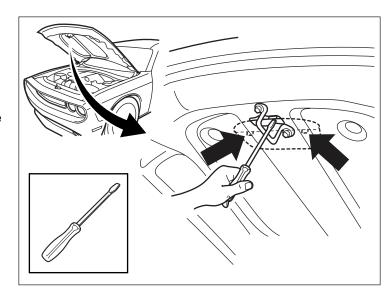
6. Lower hood down and rock the hood bezel out.
