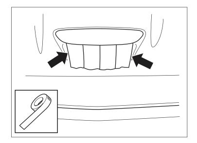
5. Remove hood bezel by prying (2) tabs, until they unsnap with a flathead screwdriver.
