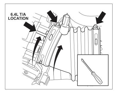
24. Install MUA hose (4) for 6.4L engine or (2) for 5.7L engine. Fit till snug, 5.7L engine shown.
