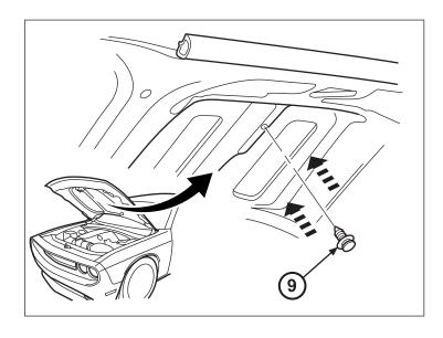
10. Align "Keyhole Slot" on hood mounted duct assembly (10) to double stud locating pin (9) and hold in place while sliding hood mounted duct tabs into hood bezel & adaptor assembly (1).
