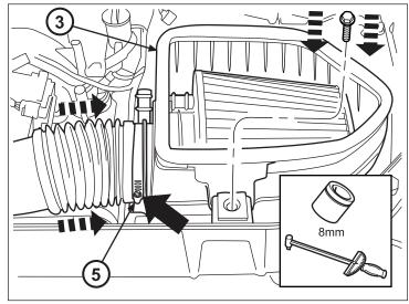
23. **FOR 6.4L MODELS ONLY**: Loosen band clamps and rotate CSD air duct clockwise rearward. Note index notch for 6.4L on airbox. Duct throttle body index will be on inboard rib. Tighten clamps when in position.
