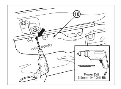
13. Insert one M6 x 30 fastener (7) into hood mounted duct assembly (10) as shown. Push to seal flush.
