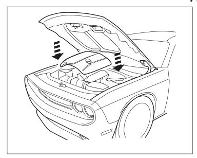
27. Close hood gently, inspect complete assembly for deformities or any mis-alignments, adjust where necessary.
