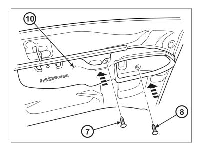
12. If necessary on (2011-2016) models, Drill 6.5 mm (1/4") hole in center stance opening of the hood mounted duct assembly (10) into the hood.
