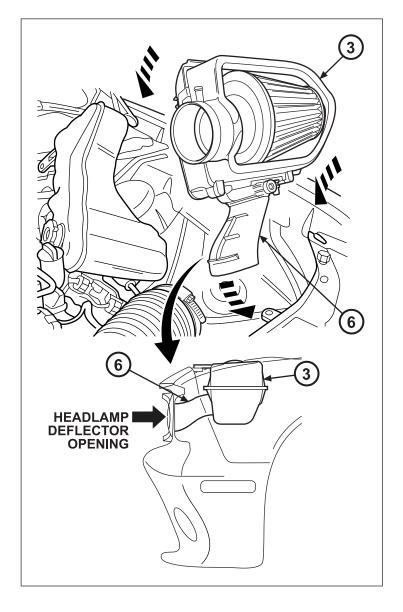
22. Reinstall airbox mounting bolt to airbox (3) with 8mm socket and torque to: 4 N.m. (35.4 in.lbs.)
