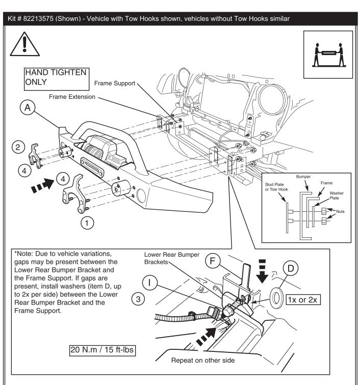
Rotate Bumper under frame extension to align lower rear bumper bracket slots to frame support hole (see frame 7) and then loosely install two tow hooks with nuts and washer plates (removed in step 5). Now loosely install bolts (item I) to handle nuts (item F). Due to vehicle variations, washers (item D) are supplied to eliminate gaps.
