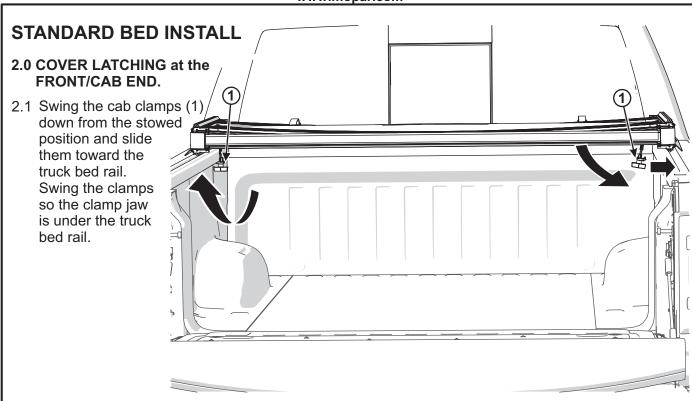
2.2 The clamp jaw must be in contact with the metal truck bed rail, **Do Not** secure to the plastic bed rail or bed cap.
