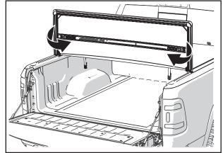
3.2 Open the tailgate, swing the tail clamps (2) down from the stowed position and slide them toward the truck bed rail.
