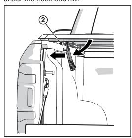
The clamp jaw must be in contact with the metal truck bed rail. **Do Not** secure to the plastic bed rail or bed cap. Check that both clamps are securely tightened to the metal bed rail.
