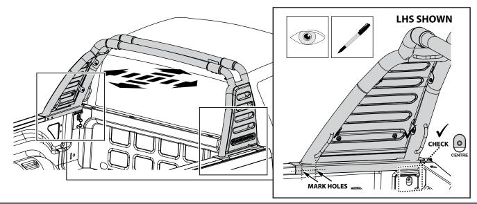
**8.** Align the Sports Bar with the front edge of the tub. Check the threaded hole in the Front Foot is centred and mark the locations of the two rear holes onto the tub with a marker. Remove bar.
