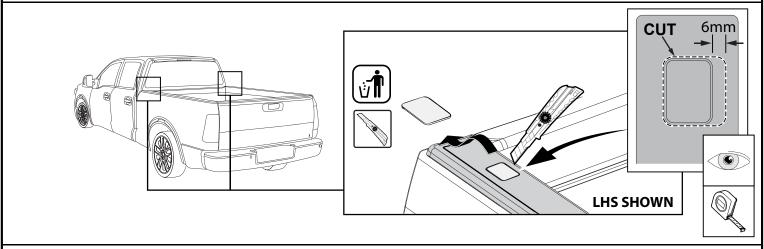
5. Using a knife carefully measure and cut out the plastic insert as shown at the front of the LHS and RHS bed rail caps to open the clearance holes inboard for the front feet of the Sports Bar.
