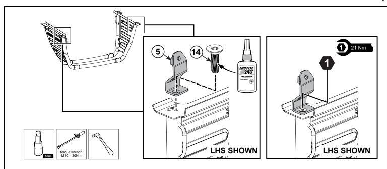
**4.** Apply loctite to the threads on the Countersunk Bolt (14) and assemble the Left Hand Side Front Foot (5) on tub rail bracket using the Countersunk Bolt (14). Tighten the bolts to the recommended torque of 21Nm. Repeat for RHS.
