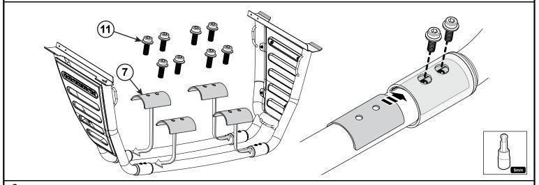
3. Slide the Joiner Plates (7) into the gaps between the plastic Joiners and the tubes and align. Secure the tubes together with the Flanged Allen Bolts (11). Do not tighten.
