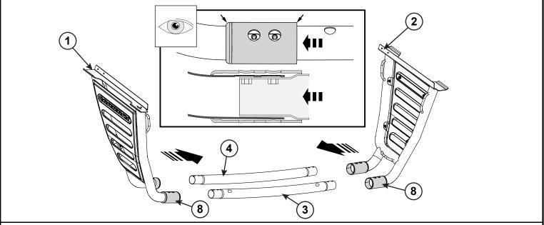
2. Assemble the Sports Bar by sliding the Front (3) and Rear (4) Tubes into the Side legs. Push the tubes into the Side legs and align the weld nuts in the tubes with the holes in the plastic Joiners (8).
