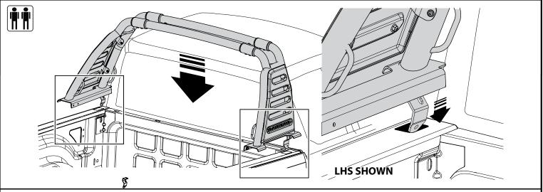
**7.** Using two people carefully lift the sports bar into position above the tub and slowly lower the sports bar front feet through the bed rail stake pockets and lower the sports bar assembly onto the tub of the vehicle.
