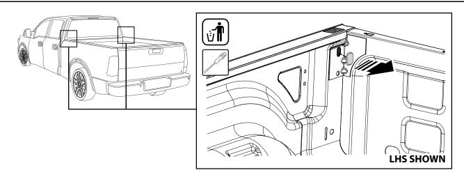
**6.** Remove and discard the LHS and RHS plastic side plugs from the tub.
