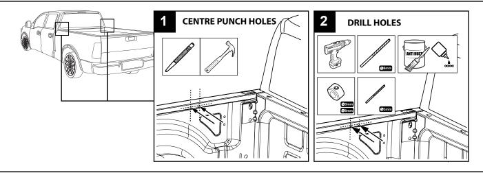
**9.** Centre punch the two marked hole positions and drill each hole with a 3mm drill bit then with an 8mm drill bit using a drill stop at 10mm. Coat exposed metal with rust inhibitor and clean up any metal swarf. Repeat for the RHS.
