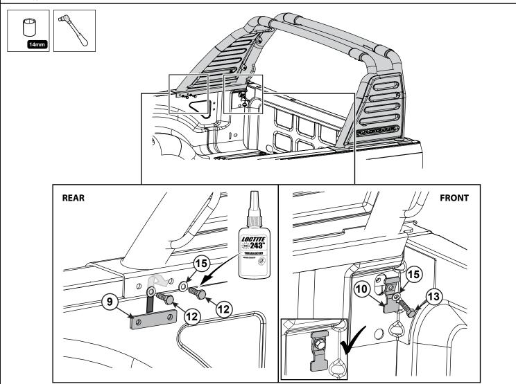
**11.** Apply loctite to both M8 bolts (13) and loosely attach the bar to the front of the tub using the Front Foot Clamp (10), M8 Bolt (13) and M8 Washer (15). Attach the Sports Bar to the rear of the tub using the Rear Foot Clamp (9) and M8 Bolt (12) and M8 Washer (15) as shown.
