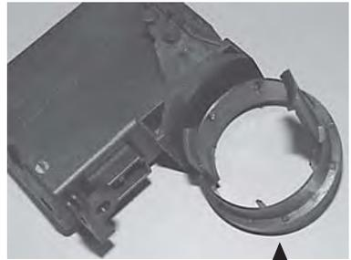
Transceiver Antenna Coil
