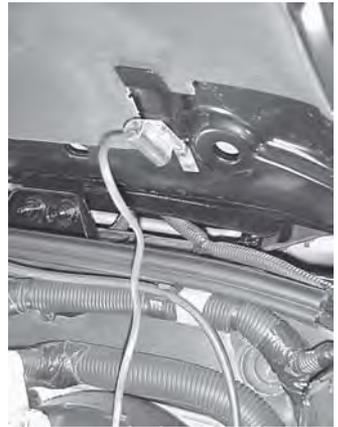
B. Using a supplied 1/4" screw, secure the ground lead from the switch to the metal cowl panel. The remaining wire will be connected later.
