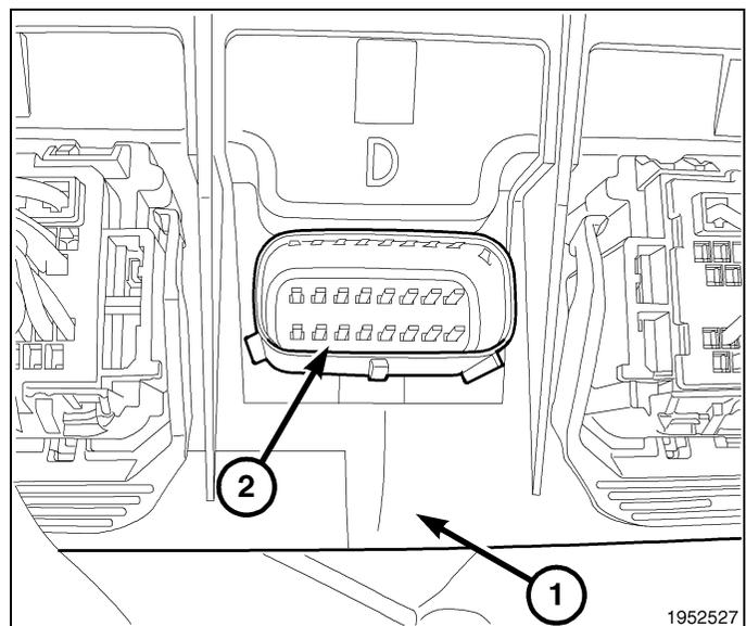
18. Route the pigtail wires down the harness to the TIPM and secure where necessary.
