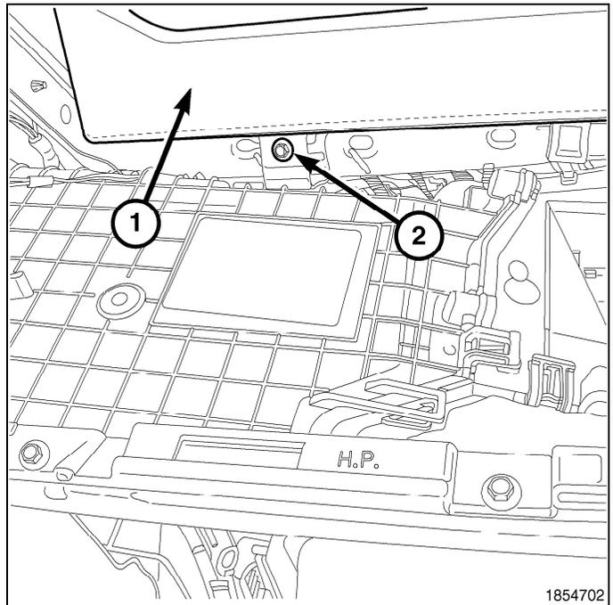
16. Engage the hinges (1) of the glove box (2) to the instrument panel.
