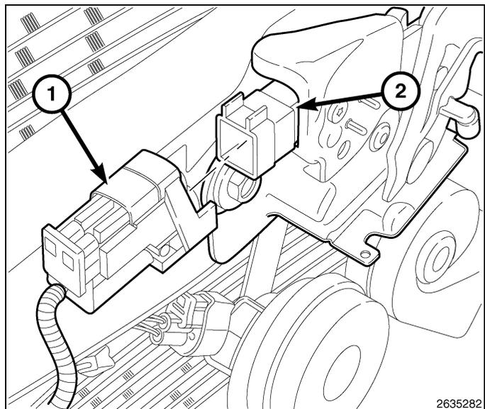
10. Route the hood switch harness (2) under the upper radiator crossmember towards the left side of the vehicle.
