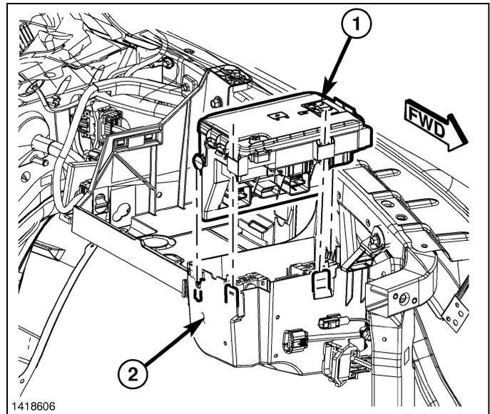
17. Disconnect the connector C4, letter D labeled on the bottom of the TIPM. Release by depressing the locking tab and rotating the connector arm outboard, until the connector is free from the TIPM assembly (1). Be certain to pull the connector straight off.
