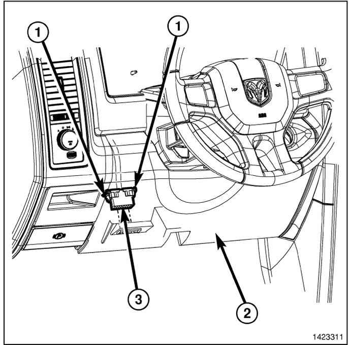
6. Install the two fasteners (2) that secure the steering column opening cover (1) to the instrument panel.
