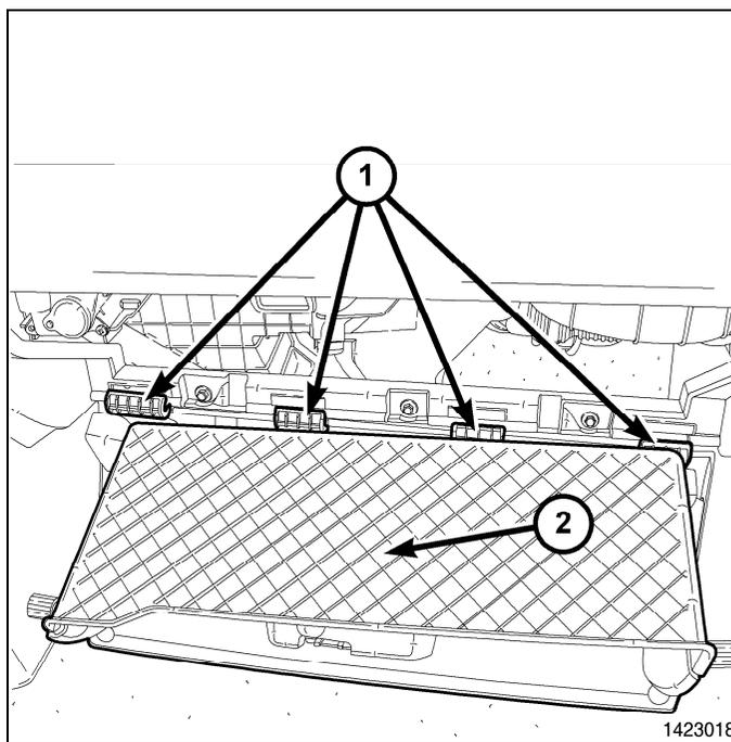
17. Press downward on the back edge of the glove box (2) and raise the glove box past the two stops (1).
