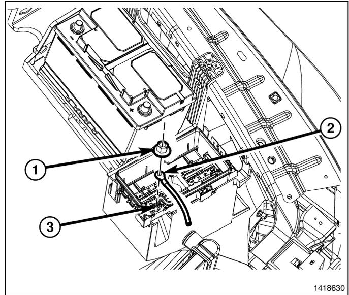
16. Grasp the TIPM (1) and rotate the assembly up to free it from its mounting bracket (3). Position the assembly upside down to access the electrical connectors located on the bottom of the unit.
