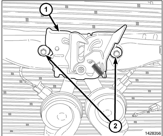
5. Disconnect the hood latch cable (1) from the hood latch (5) and remove the latch.
