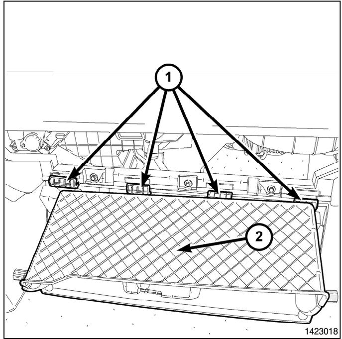
4. Through the glove box opening remove storage bin fastener (2) located at the back of the storage bin (1).
