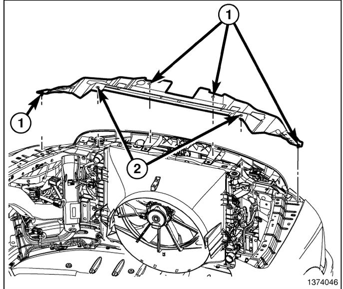
3. Using a grease pencil or equivalent, mark the position of the hood latch (1) on the upper radiator crossmember.
