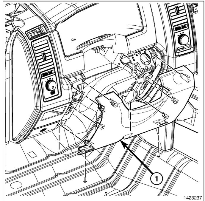
5. Install the Data Link Connector (3) to the steering column opening cover (2) by pushing the connector through the opening on the back side of the cover and fully engaging the lock tabs (1) of the connector.
