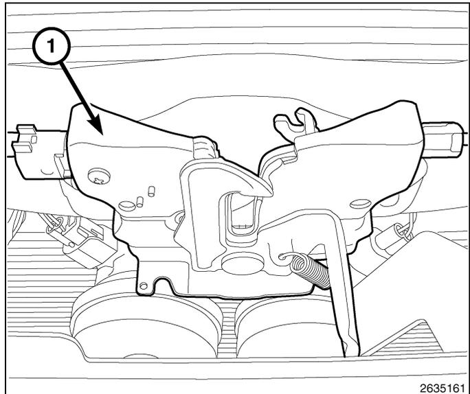
**NOTE:** There may be an unused factory installed hood switch harness taped back on the existing vehicle harness located behind the radiator just below the upper radiator crossmember. If present, detach it, route it under the radiator crossmember through to the hood latch assembly and connect. If the factory hood switch harness is not present, follow steps 9-32.
