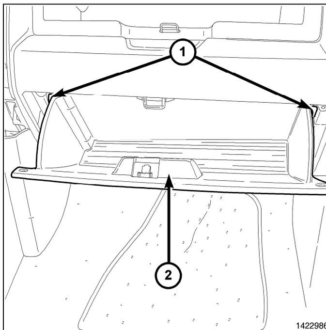
3. Disengage the glove box hinges (1) from the instrument panel and remove the glove box (2).
