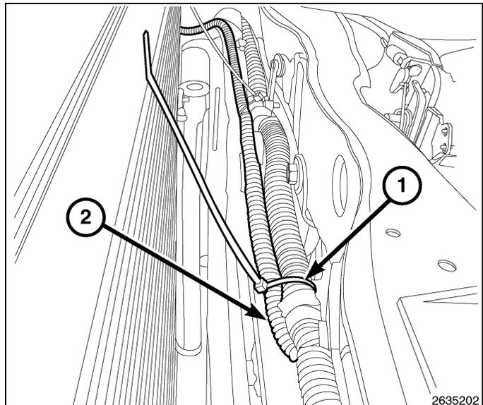
12. Route the hood switch harness (1) under the radiator mounting bracket towards the inner left fender. Secure the hood switch harness (2) as necessary to the existing vehicle harness using the tie straps (1) included in the kit.
