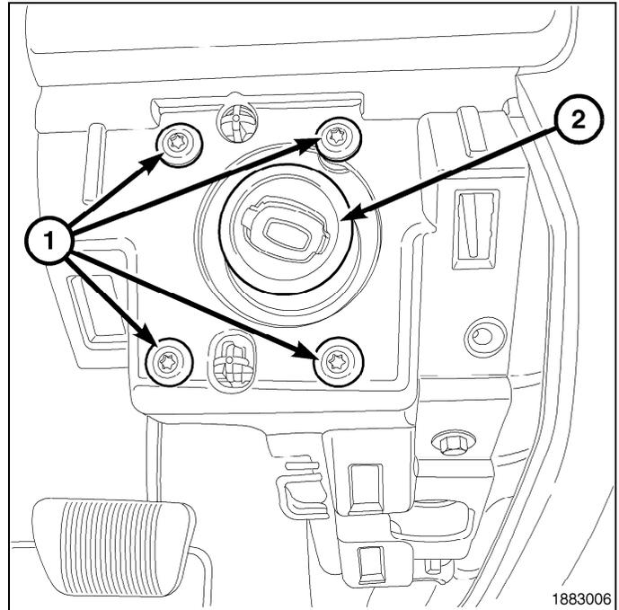
4. Position the steering column opening cover (2) to the instrument panel and fully engage the retainer clips to the instrument panel.
