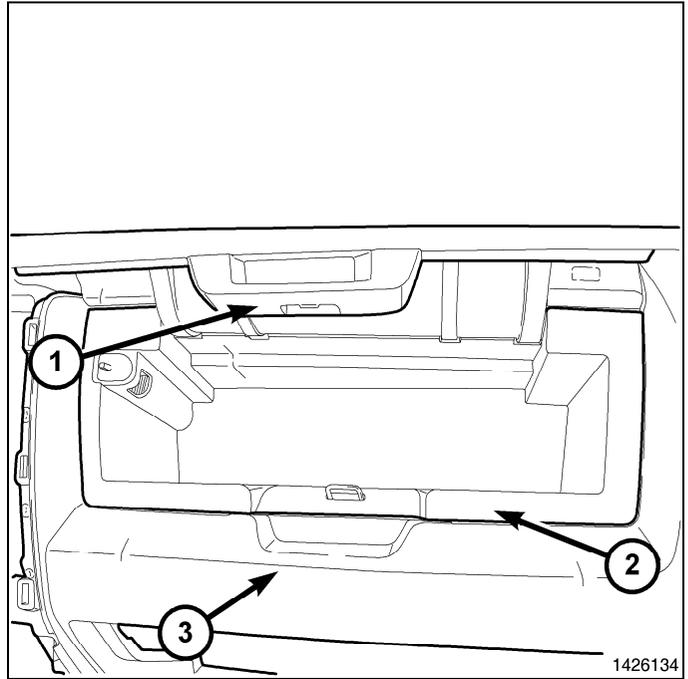
15. Through the glove box opening install the storage bin fastener (2) at rear of storage bin (1).
