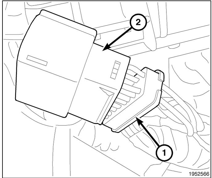
20. Remove the weather seal from the rear of the connector.
