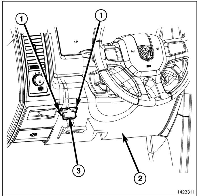
4. Using a trim stick C-4755 or equivalent, release the retainer clips that secure the steering column opening cover (1) to the instrument panel and remove the cover.
