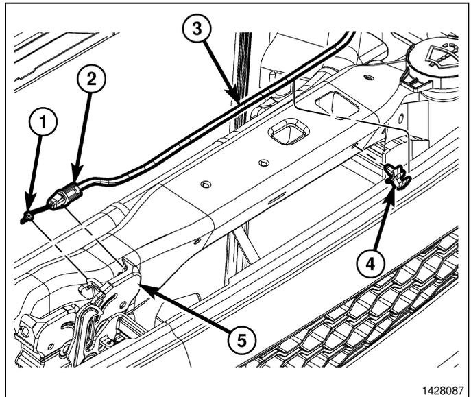
6. Connect the hood latch cable to the hood latch assembly (1).
