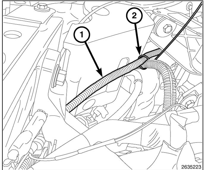
13. Remove the ground retainer (1) from the inner left fender (3).
