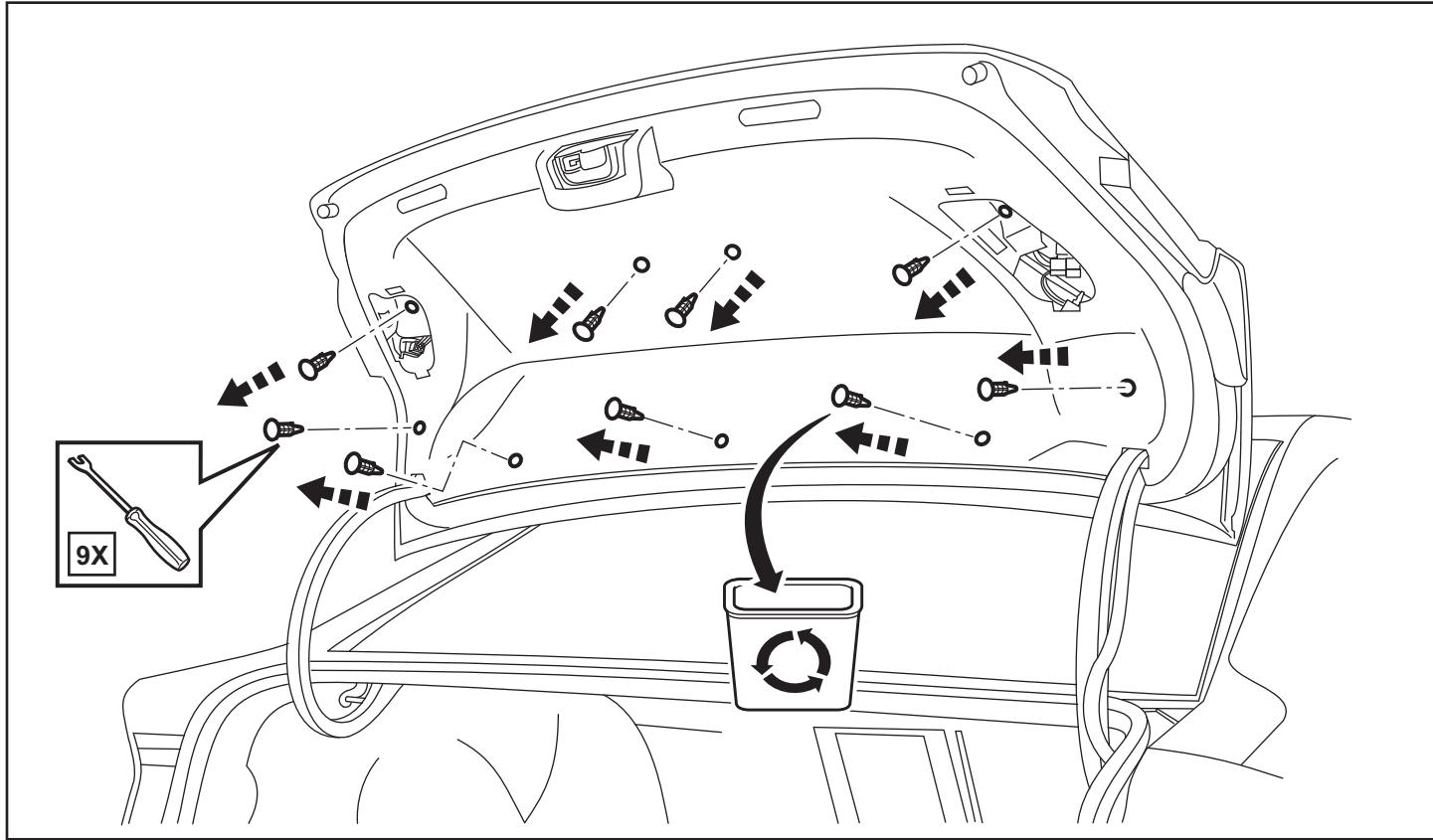
6. Carefully remove the trunk liner panel.
