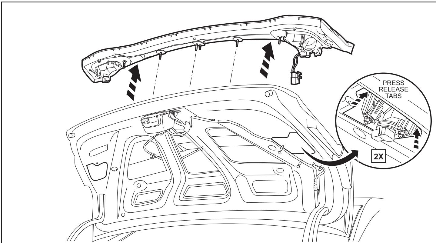
9. Install the new rear light applique assembly into the trunk lid. Be sure to feed the 6-way connector plug through properly on the right side opening.
