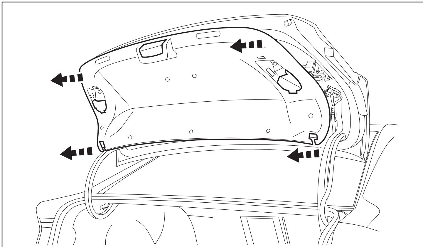
7. Remove five (5) 8mm nuts across the inside center of the trunk lid. Loosen the four remaining 8mm nuts on the far right and left side of the lid without fully removing. Disconnect the 6-way plug on the right side of the trunk lid.
