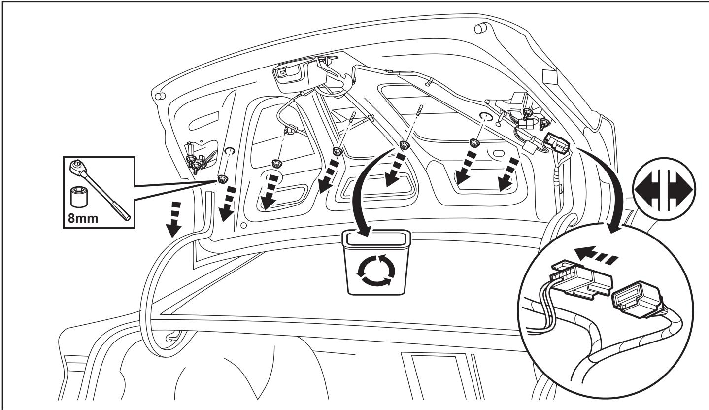
8. Press in on the two release tabs behind the lamp assemblies on both sides of trunk lid. Carefully remove the rear light applique assembly from the trunk lid.
