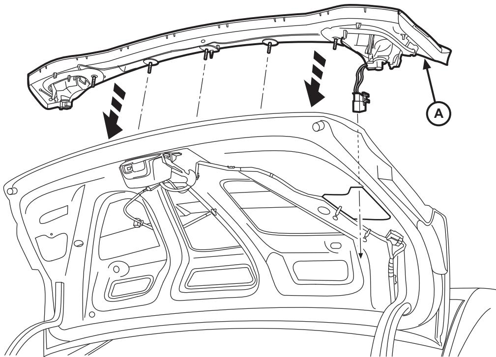
10. Reinstall five (5) 8mm nuts and retighten four (4) 8mm nuts inside the trunk lid. Reconnect the 6-way plug on the right side of the trunk lid.
