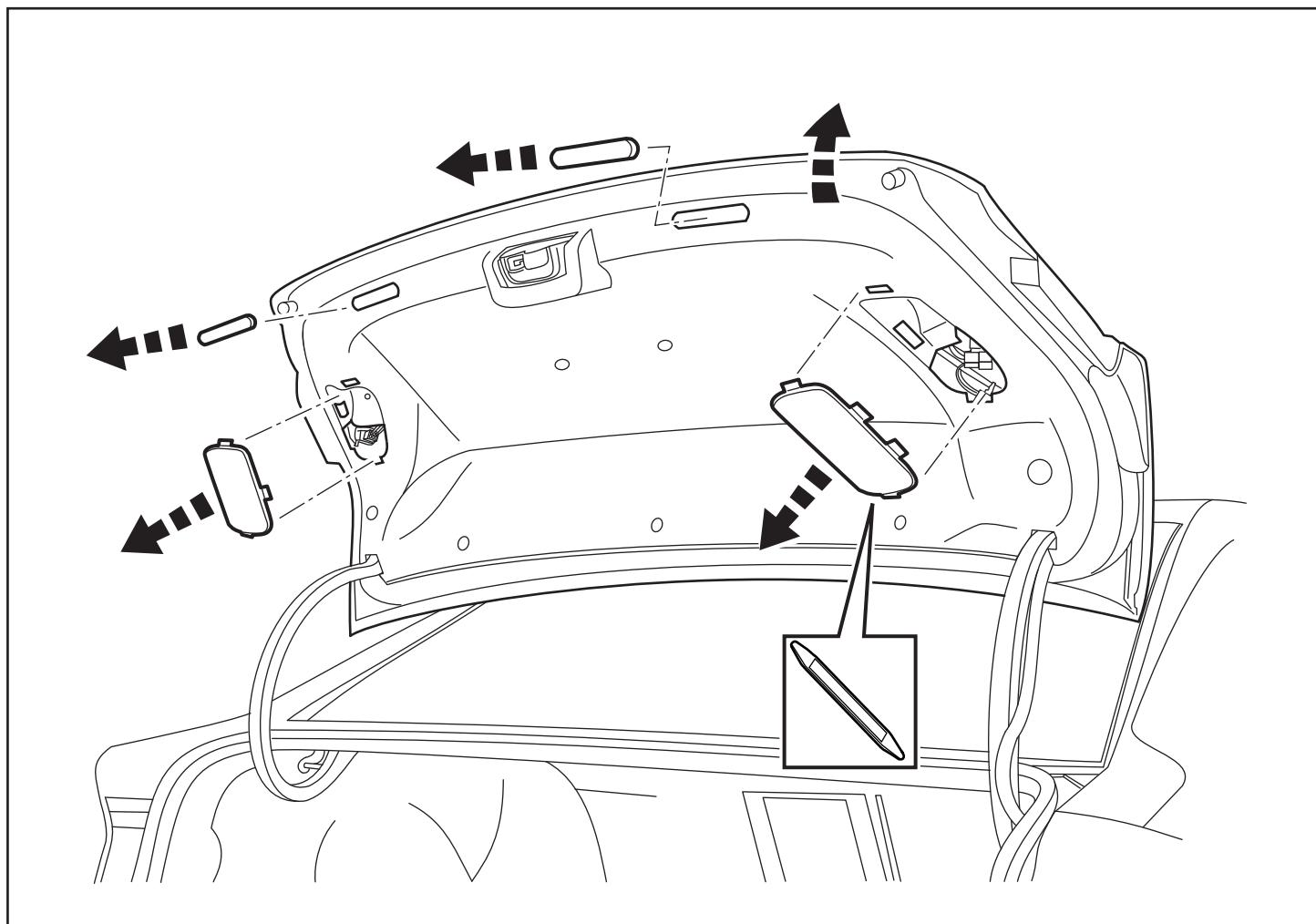
5. Use a pry tool to remove the nine (9) press clips from the trunk liner panel.
