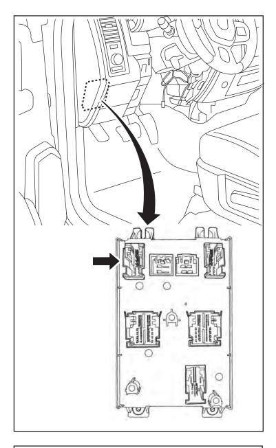
16. Press in on the release tabs at the back of the connector and slide the plug out from the outer casing.
