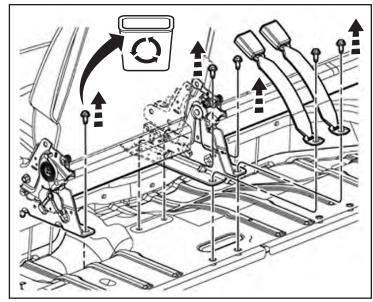
30. Remove the front fasteners. Lift the seat assemblies up and separate three (3) cab hooks from the rear loops. Remove the seat assembly from the vehicle.
