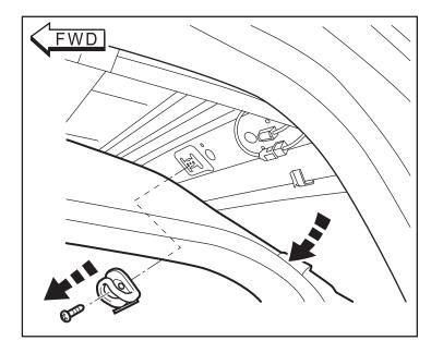
46. Position the Antenna Module (D) above the rear window. Secure in place by pressing two (2) christmas tree fasteners (J) into the mounting holes provided.
