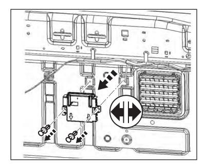
44. Place the new RF Hub Module (C) into position. Secure the RF Hub Module to the wall with two (2) push pin fasteners provided (F) and reconnect all harness connectors.
