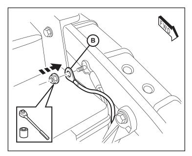
10. Locate the rubber grommet at the back of the engine compartment. Cut away the end of the access nipple and feed the end of harness (B) through to the inside driver footwell. Apply RTV sealant to the hood switch wiring convolute and pull the wiring into the nipple to seal the wiring at the nipple.
