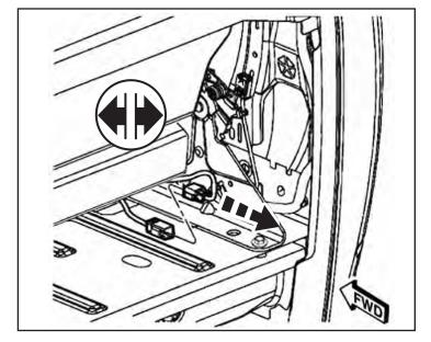
28. Remove one (1) bolt attaching the center shoulder belt to the retractor. Position the shoulder belt out of the way.
