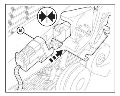
7. Route the switch harness (B) under the upper radiator crossmember and over towards the driver side along the existing vehicle harness. Secure with cable ties (E).
