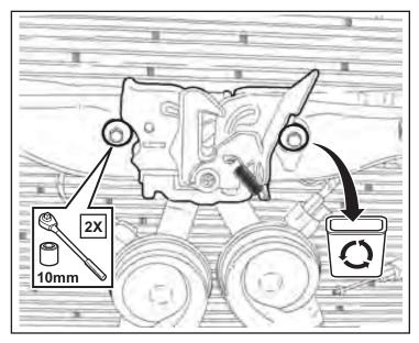
4. Disconnect and remove the hood latch release cable. Remove the hood latch assembly.
