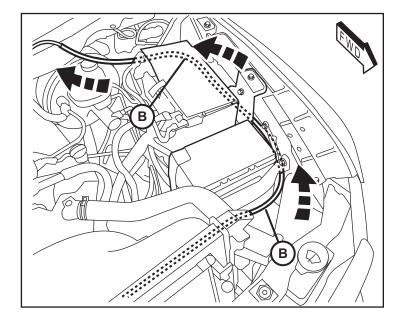
9. At the fender edge next to the battery, remove the existing ground wire hex nut. Position the ground ring terminal from the main harness (B) and reattach the nut to secure.
