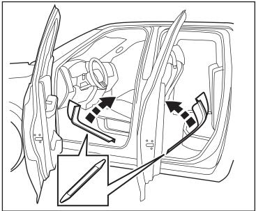
36. Release all retaining clips and remove lower trim panel.
