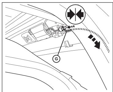
48. Route the cable (G) down along the C-pillar and secure every 150mm with Strap Tape (I) as shown.
