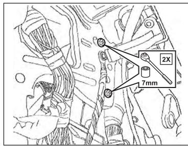
14. Loosen the one (1) 7mm amplifier bracket mounting screw located at the top of the bracket. Remove the amplifier and bracket assembly from the vehicle.
