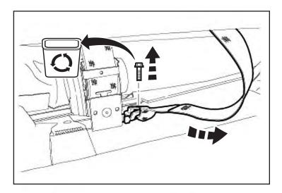
29. Remove the rear outer bolts, rear inner bolts and buckles as necessary.
