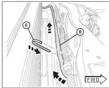
8. Route the switch harness (B) under the driver side radiator mounting bracket. Carefully feed the harness back towards the rear of the engine compartment by routing it behind and under the fuse box and the battery. Secure with cable ties every 100mm as necessary (E).
