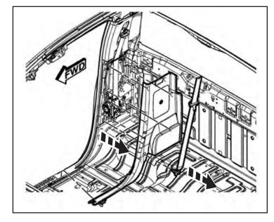
34. Use a trim stick to remove the seat belt turning loop cover. Remove the turning loop bolt. Remove the upper trim panel and release any retaining clips.
