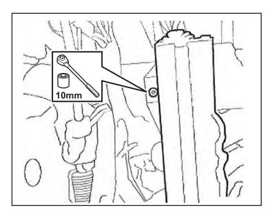
15. Locate the BCM up behind the left side of the dash. Locate and remove the top left connector from the BCM as indicated.
