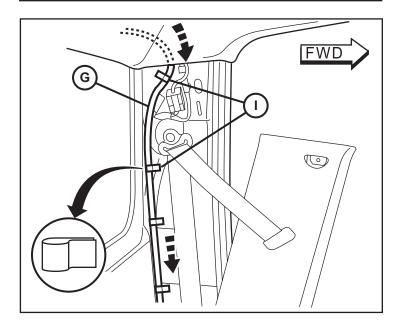
49. Plug the jumper cable (G) into the RF Hub module (C) behind the rear seat. Secure the cable along the rear wall every 150mm with Strap Tape (I).
