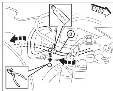
11. Remove two fasteners at the bottom of the trim panel under the steering wheel and carefully pry off the hood release latch. Disconnect the data link connector and pry off the trim panel. Pull the Switch Harness (B) through to the inside footwell.
