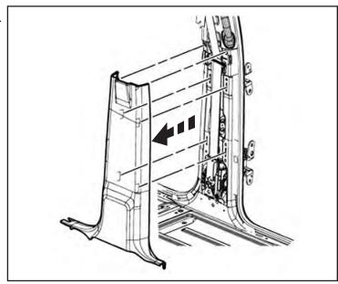
37. Use a trim stick to remove the two fastener covers at the grab handle. Remove two (2) fasteners from the grab handle and remove the grab handle from the B-pillar. Remove the seat belt turning loop cover and remove the turning loop bolt. Use a trim stick to release all retaining clips and remove the trim panel from the B-pillar. Remove the seat belt from the trim panel and remove the panel from the vehicle.
