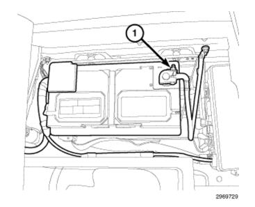
• Disconnect and isolate the negative battery cable (1).
